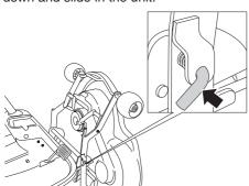
2 Replace the cutting height stay and the belt. Tension the belt with the belt adjuster.
